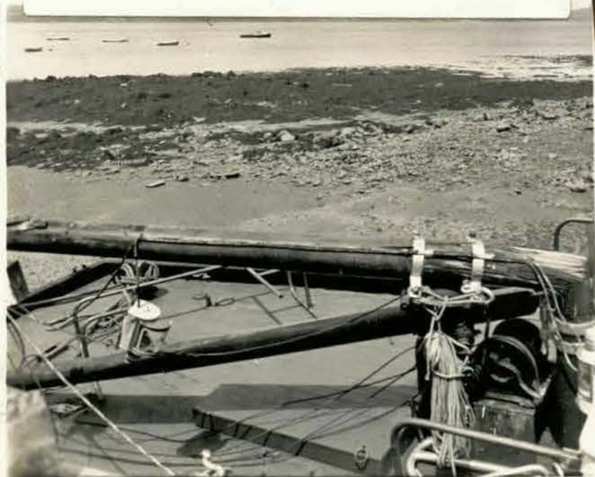
Neg. No. DB 9347 Dispo.L.. HQ.. Dest.. Photog. Ellis Dept. Cdr. Damage to harbour craft. View showing break in the spar.
