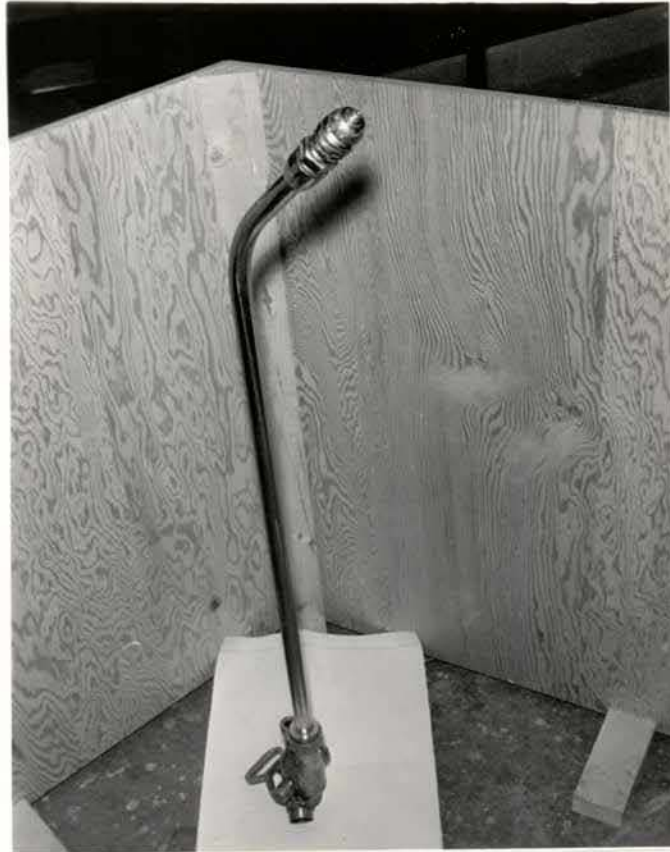
DB 12056 Dispo: L..HQ..Dest.. Photog. Maheux Dept. Training Rockwood nozzle and applicator.
