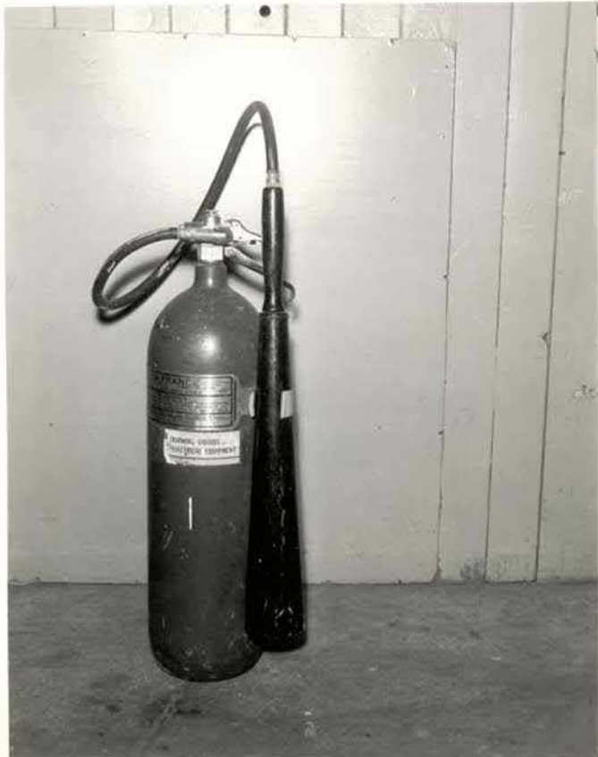
DB 12057 Dispo: L..HQ..Dest.. Photog. Maheux Dept. Training CO2 Fire extinguisher
