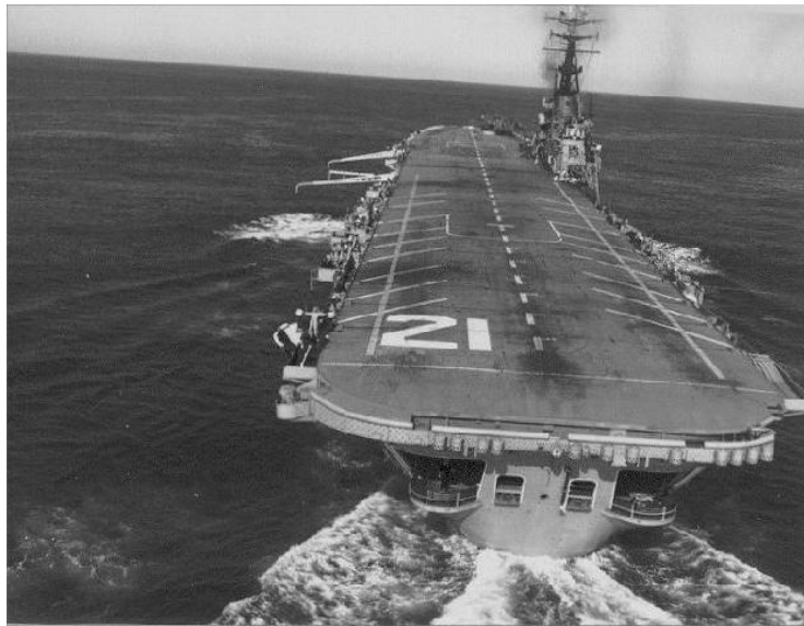
----and as seen by a pilot on final approach. Note the "batsman" on the after port sponson.
