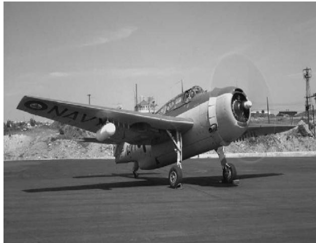
The Grumman Avenger, fondly referred to as the "Turkey", in its ASW configuration after conversion from its wartime TBM role.
