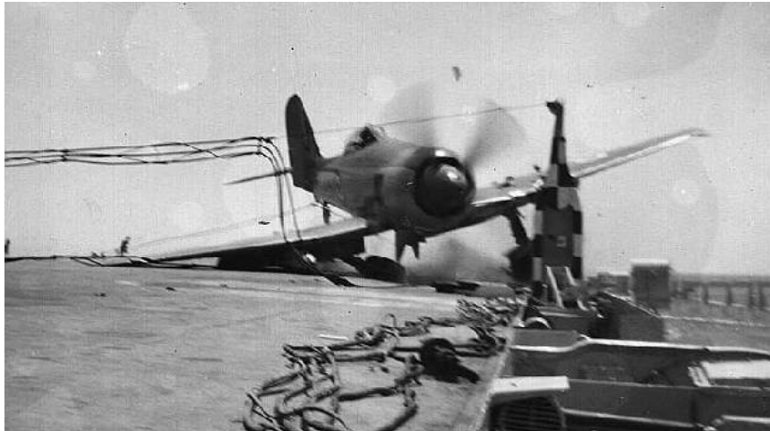
The Fury that didn't make it. Note the crumpled oleo and the broken wire barrier. With luck it will end up in the sponson rather than the water.
