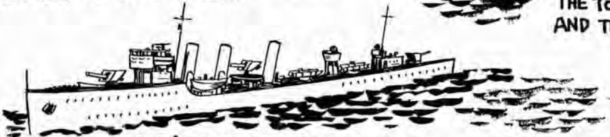
'L, M, N, R, & S' CLASS DESTROYERS OF WORLD WAR I - 3 4 IN. GUNS, 4 TORPEDO TUBES, 29-36 KNOTS...
