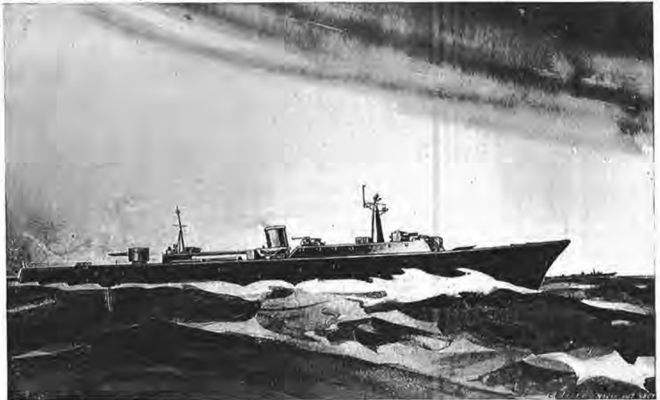
Above is an artist's conception of the RCN anti-submarine escort vessel, working drawings of which are now being prepared. It is expected that keels for three of the new ships will be laid down at the end of the year or early in 1950. The escort vessels will have steel hulls and aluminium superstructures and bridges and will be driven by steam turbines. Accommodation will be provided for a crew of more than 250. ("Crowsnest," July 1949.)
