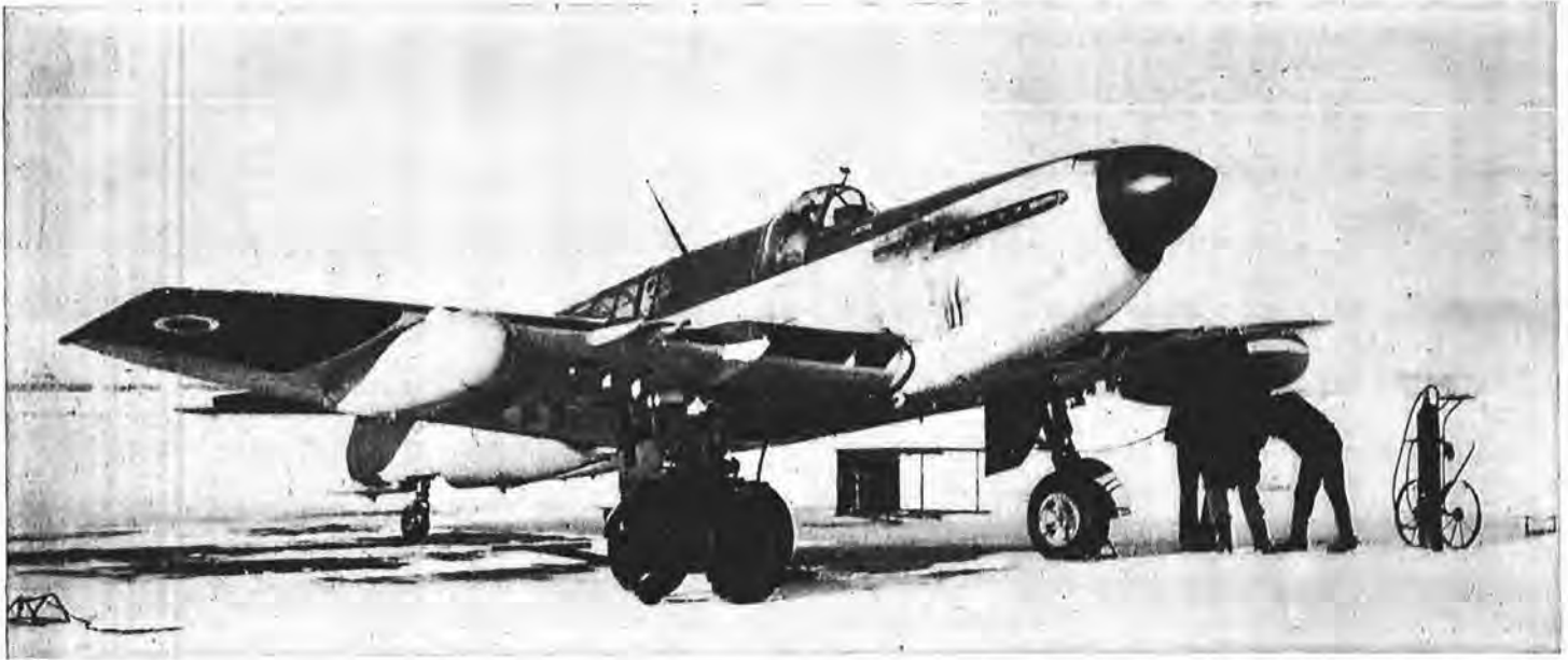
Cold starting tests being carried out on the Firefly 4 at Watson Lake. When the mercury is out of sight, this is not the pleasantest of work.
