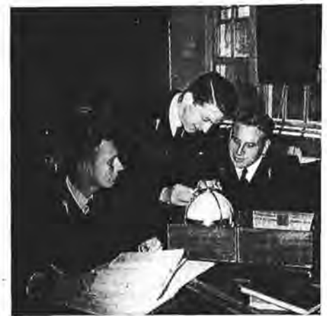
As part of their three-week course in the Navigation Direction School at HMCS "Stadacona," Cadets RCN (R) learn the use of the star globe, a device for identifying stars. From left to right are Cadets W. E. Ogden, Toronto; L. Lemieux, Montreal, and G. R. Todd, Wolfville, Nova Scotia.
