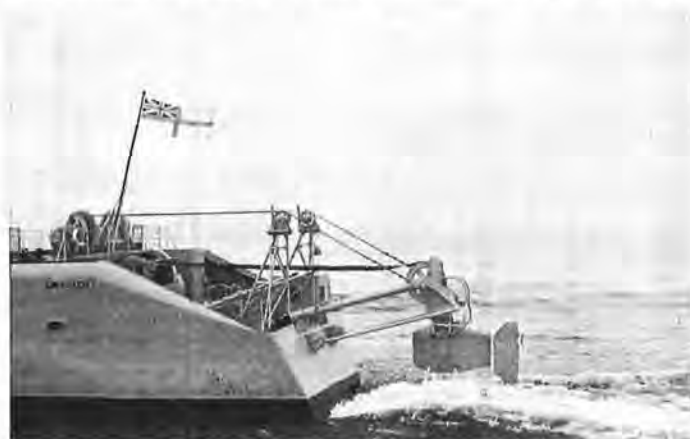
Figure 2: Variable depth sonar installation in HMCS St. Laurent. (E-65750)
