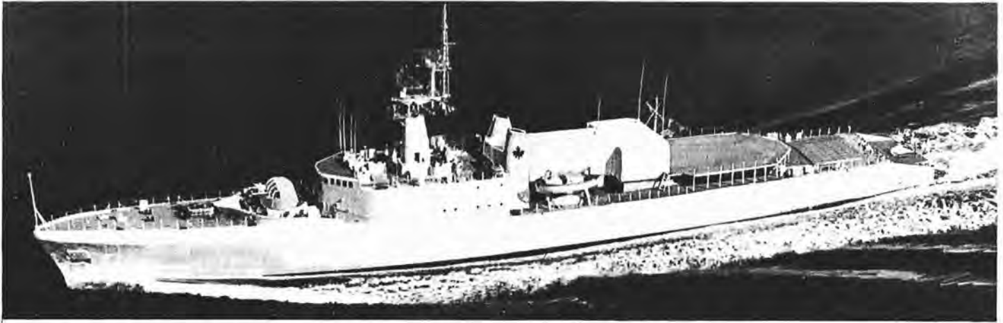
Figure 6: Artist's conception of converted St. Laurent class destroyer escort, with helicopter platform, hangar and variable depth sonar. (CN-6407)
