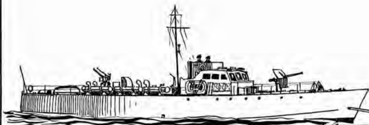
FAIRMILE TYPE 'A' CONVERTED AS A MINELAYER WITH 6 GROUND MINES AND FUNNEL REMOVED
