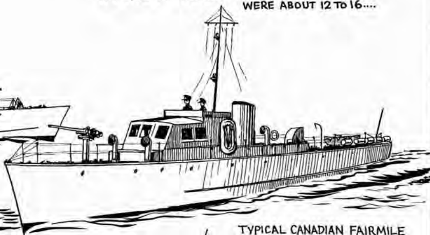
TYPICAL CANADIAN FAIRMILE (TYPE 'B'), USED EXTENSIVELY BY THE R.C.N. ON COASTAL A/S PATROL. ARMED WITH DEPTH CHARGES...
