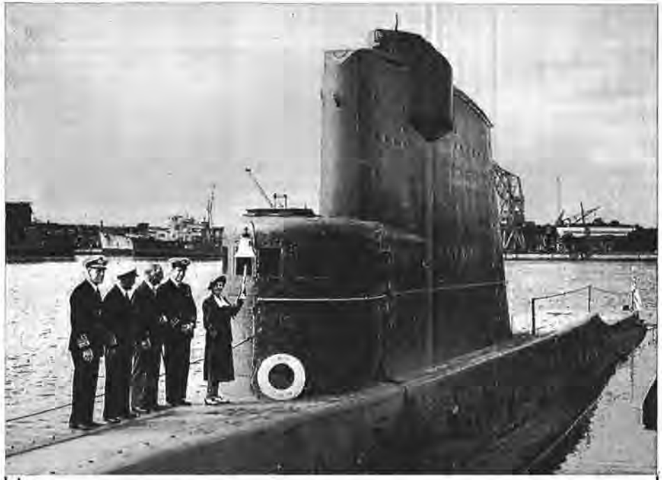
HM Submarine Turpin, above, presents a startling effect following her conversion to withstand atomic bomb attack. In an extensive rebuilding job, the Turpin had her superstructure and hull "ironed out" to offer a minimum of resistance to atomic blast. A streamlined conning tower masks the periscope, radar mast and other navigational and operational aids, while forward of it is what appears to be a wheelhouse equally streamlined. Originally launched in 1944, the Turpin was launched recently for the second time, with Lady Tovey, wife of Admiral of the Fleet Lord Tovey, officiating. Lady Tovey is shown holding the submarine's bell. (United Kingdom Information Office Photo).
