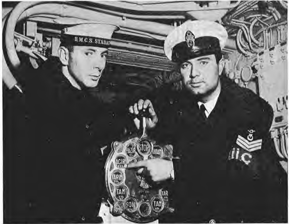
"Stop" apparently means the same thing to both Turkish and Canadian engineers, although the meaning of the other markings on the engine room telegraph of one of the Bangors turned over at Sydney to the Turkish Navy might not be entirely clear to RCN personnel. (HS-50828)
