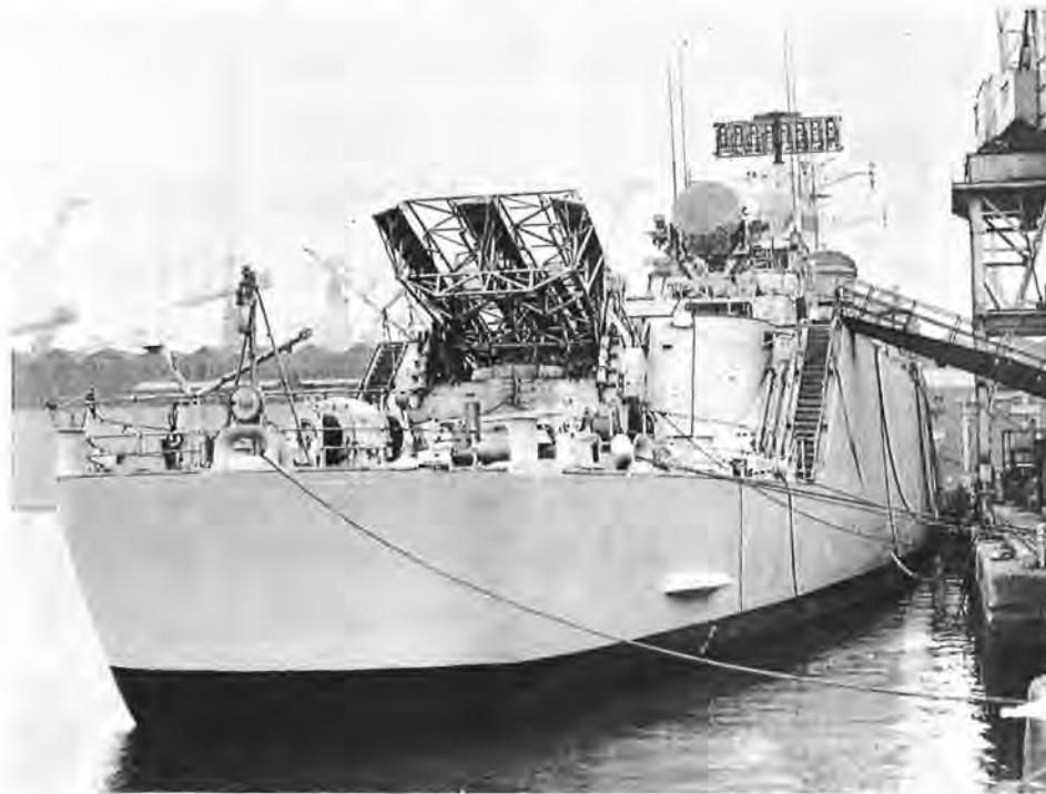
HMS Devonshire, the Royal Navy's first guided missile destroyer, is shown in port after completing sea trials with the Seaslug anti-aircraft guided missile. Behind the missile launchers is the radar beam rider which guides the missile onto its target. (British Information Service)
