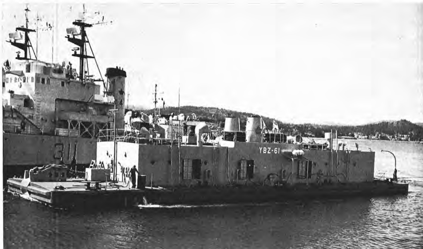
Housemaid of the RCN's Pacific fleet, the YBZ-61 is, in effect, a huge vacuum cleaner whose job is to vent, clean and gas-free the fuel tanks and bilges of warships. She not only saves time, man hours and money, but makes a messy and unpleasant job much easier to tackle. The YBZ-61 is shown at work alongside the ocean escort Stettler. (E-76131)
