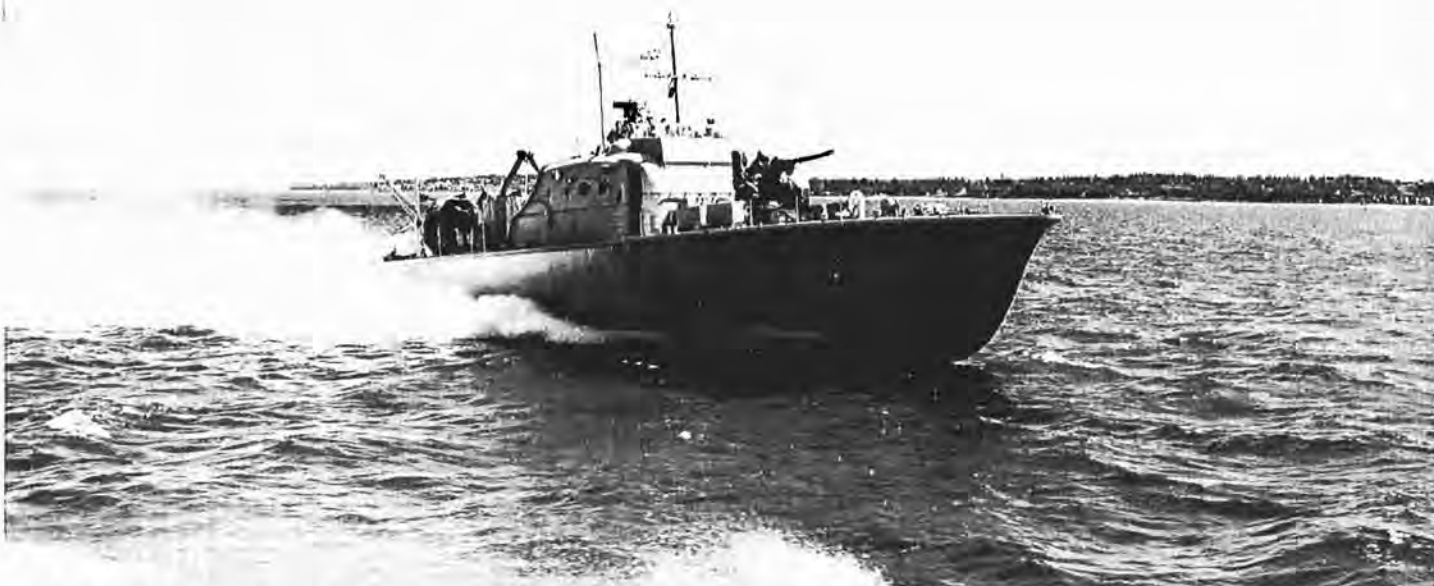
Is this, as her builders believe, the world's fastest warship? HMS Brave Borderer, first of a new class of fast patrol boats (convertible torpedo/gunboats), exceeded 50 knots on trials. Powered by three Marine Proteus gas turbine engines, developing 10,500 horsepower, she is of composite aluminum and mahogany construction. She and her sister ship, Brave Swordsman, were designed and built by Vosper, Limited, Portsmouth. (Photo from Bristol Siddeley)
