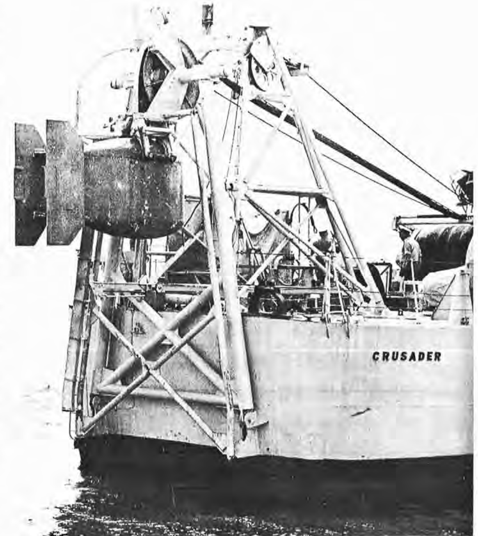
An important scientific achievement, made public early in 1960, was the development of practical variable depth sonar. Shown here is the final experimental equipment used on board HMCS Crusader before the apparatus went into production. RCN ships are being equipped with the new device. (CN-5071)
