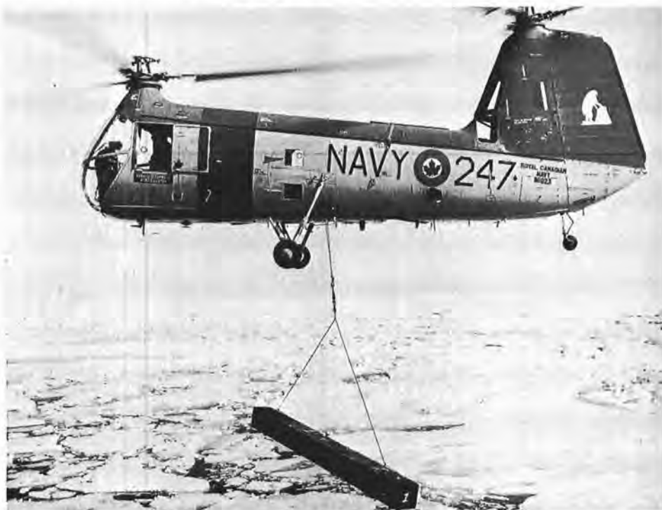
The HUP heads shoreward with a packaged 90-foot antenna mast. (LAB-958)
