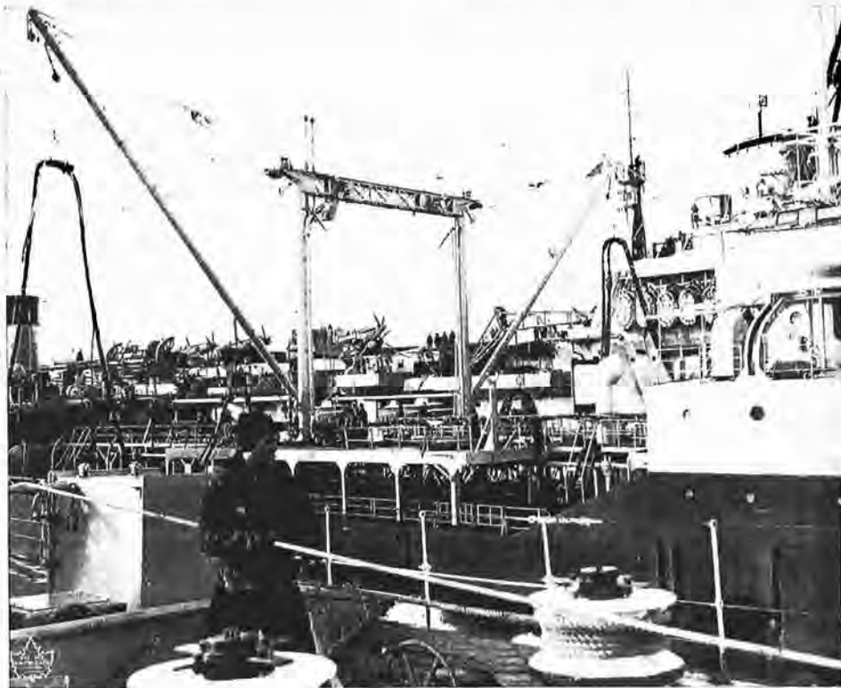
Two ships, HMCS Nootka (from which the photo was taken) and HMS Theseus, fuel at the same time from the Royal Fleet Auxiliary Wave Knight in the Yellow Sea during a Korean patrol. The fuelling operation is routine stuff for the ships of the UN fleets. The employment of fleet tankers and supply ships enables them to spend far longer sustained periods at sea than would otherwise be possible. (NK-527).
