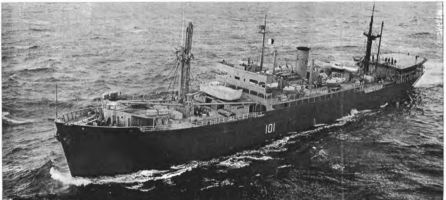
HMCS Cape Breton (100) is the escort maintenance ship based at Esquimalt. She is similar in most respects to the Cape Scott (101), based at Halifax. Note the helicopter platform aft and the heavy handling gear. (E-53746; DNS-34901)
