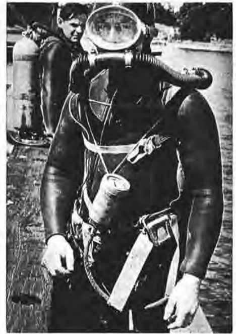
PO R. J. Thompson and Ldg. Sea. W. E. Nehring in July 1963 dive the first prototype computer at the RCN's Clearance Diving Establishment at Colwood, near Esquimalt. The computer senses the inlet pressure of the breathing apparatus and indicates the time required for an ascent to the surface to avoid the bends.
