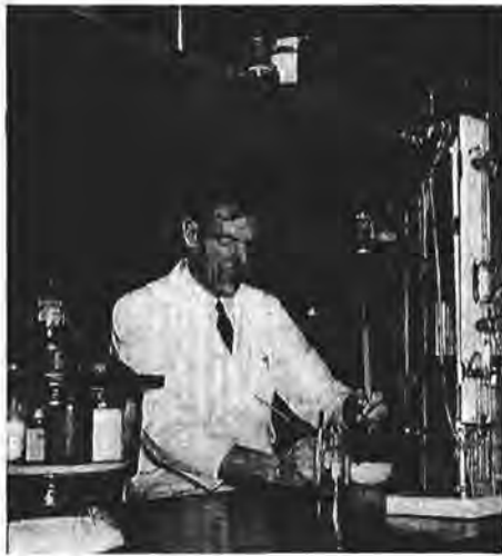
Petty Officer Ivan Wright is shown working at an automatic burette, used for titrating substances. Here he is checking the alkalinity of a fluid for clinical use. (E-10370).
