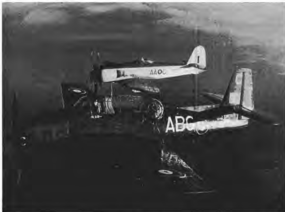
These are the two types of operational aircraft employed by the Royal Canadian Navy. In the foreground is a Grumman Avenger, an American-built aircraft modified in Canada for specialized anti-submarine duties. The other aircraft is a Sea Fury fighter, one of the world's fastest propeller-driven planes. Two RCN squadrons are equipped with Avengers and two with Sea Furies. (DNS-3898).
