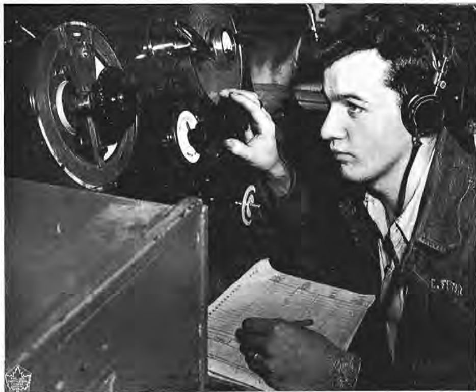
A picture of concentration is AB Ed Fetter as he operates a direction finder on board HMCS Athabaskan . Wartime W/T operators will appreciate this photo, which shows the improvements made in D/F sets as compared to the type on which they used to struggle to get bearings. (AN-146).
