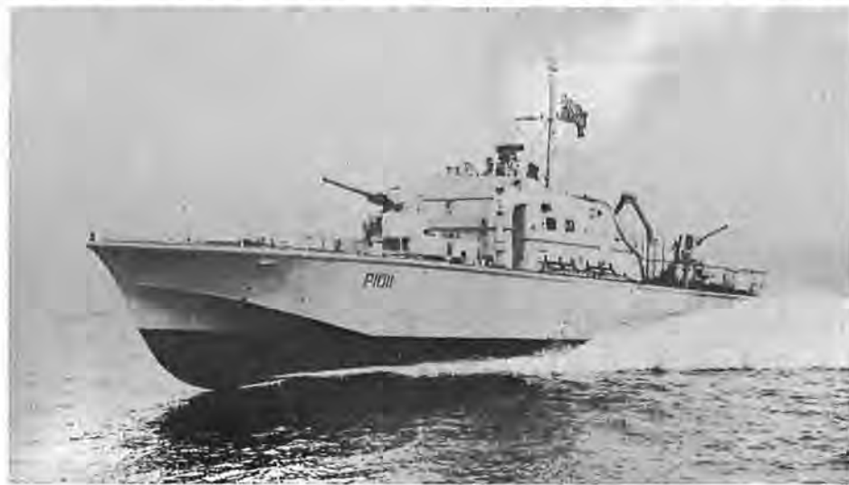
Powered by three gas turbines, HMS Brave Borderer , first of two Brave class fast patrol boats ordered by the Royal Navy, attained a speed of over 50 knots during trials in January. (Fifty knots equals about 57.5 land miles per hour.) A sister boat, Brave Swordsman , will be ready for service later this year. The craft can do duty either as motor torpedo boats or motor gunboats. (Photo from U.K. Information Office.)
