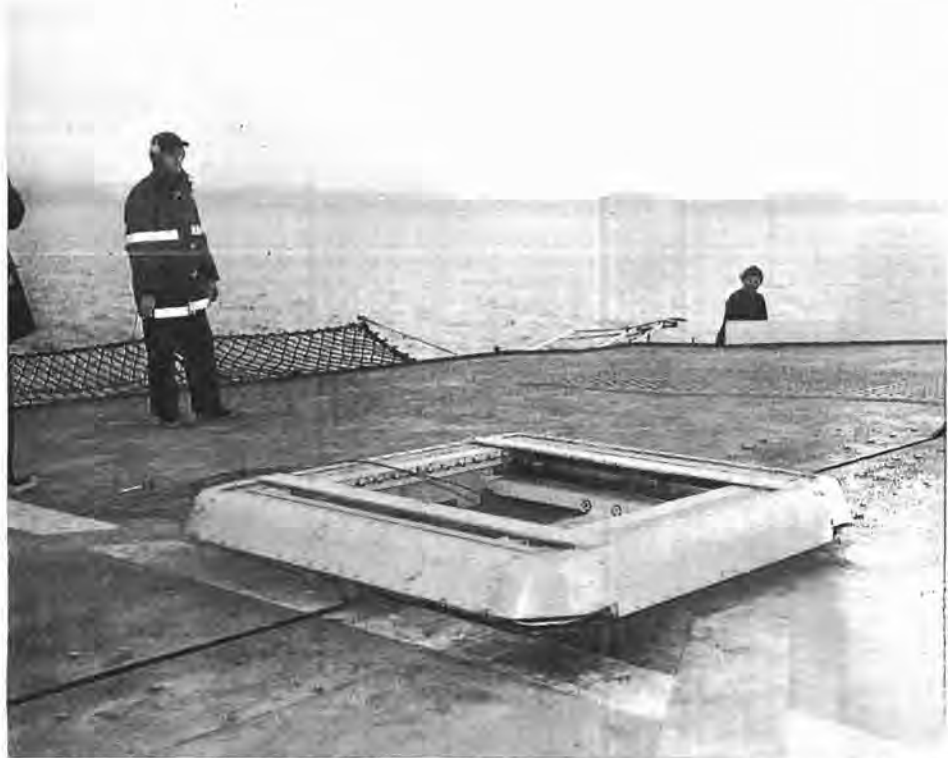
This is "beartrap", a rapid securing device, which, with the coiled haul-down cable, lies ready for the landing operation. Flight deck personnel will grab a messenger cable from the helicopter. (HS-75928)
