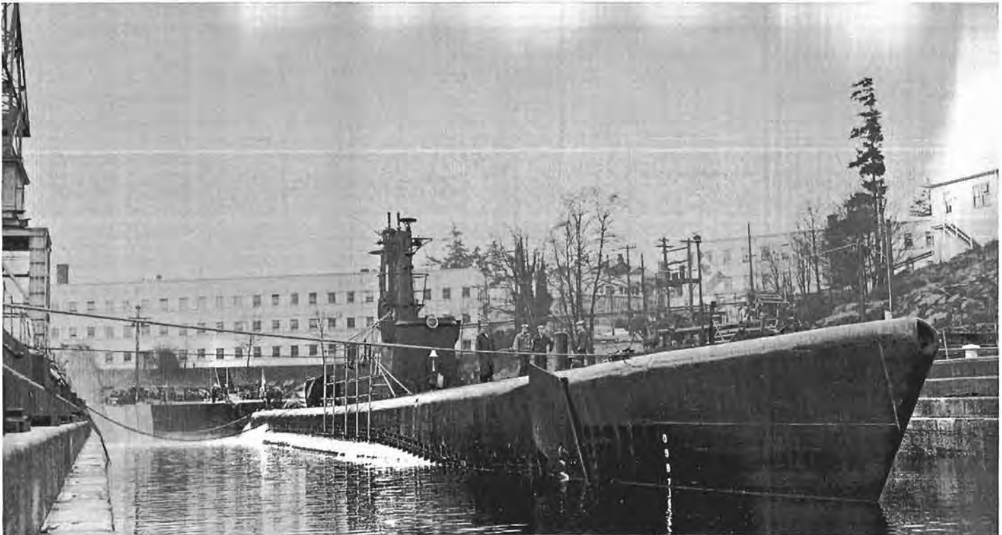
Heavy lines control the submarine Grilse as she enters the historic dry dock of HMC Dockyard, Esquimalt. After completion of a minor refit the submarine returned to fleet duties with the Pacific Command. (E-79625)
