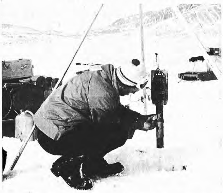
A bathythermograph slide is inserted before recording water temperature at varying depths. In the background is Vanhauen Pass, a valley which links Otto and Hare Fiords off Nansen Sound.
