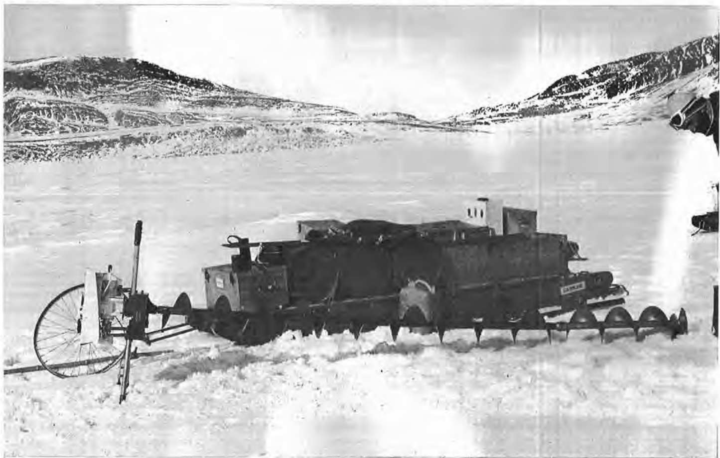
An ice auger is unloaded preparatory to bathythermograph operations off Nansen Sound. The wheel-like odometer at the rear of the sled permits the exact measurement of distance travelled.
