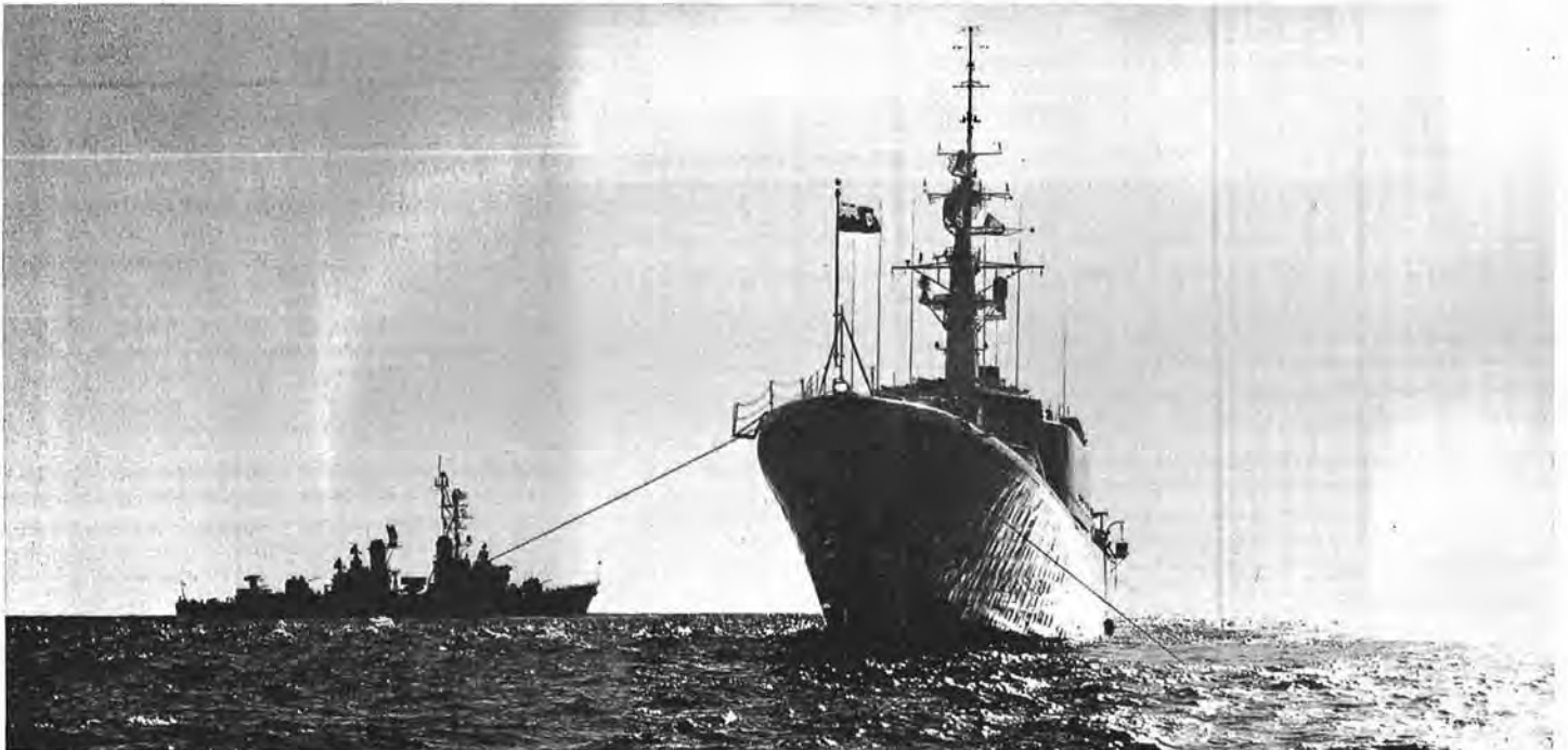
Steadied in position by mooring lines, HMCS Fraser awaits the impact of the blast from a 500-ton TNT explosion during tests in Hawaiian waters early this year. (O-19530-79)
