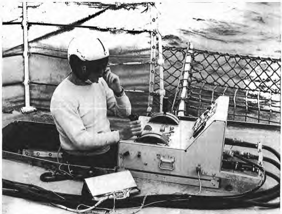
Amid multi-wired cables, the landing control officer prepares to haul down the tethered Sea King. The LCO is constantly in radio voice contact with the helicopter pilot. (CN-6826)
