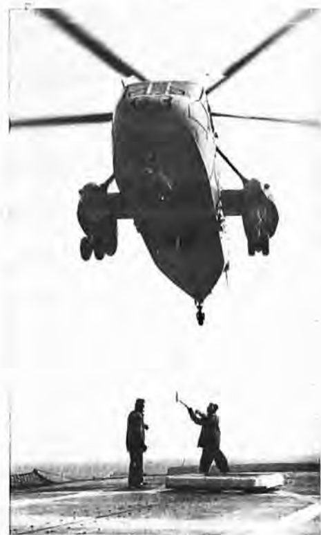
A flight deck crewman grounds the messenger while the other prepares to connect the haul-down cable. The Sea King hovers about 50 feet above the deck. (DNS-33897)
