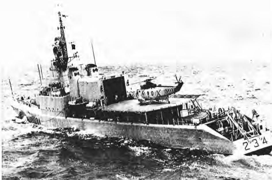
Beartrap jaws grip the Sea King's probe, clamping the 9½-ton "chopper" firmly on deck. The helicopter thus is poised for centring and shifting into the hangar. (CN-6823)
