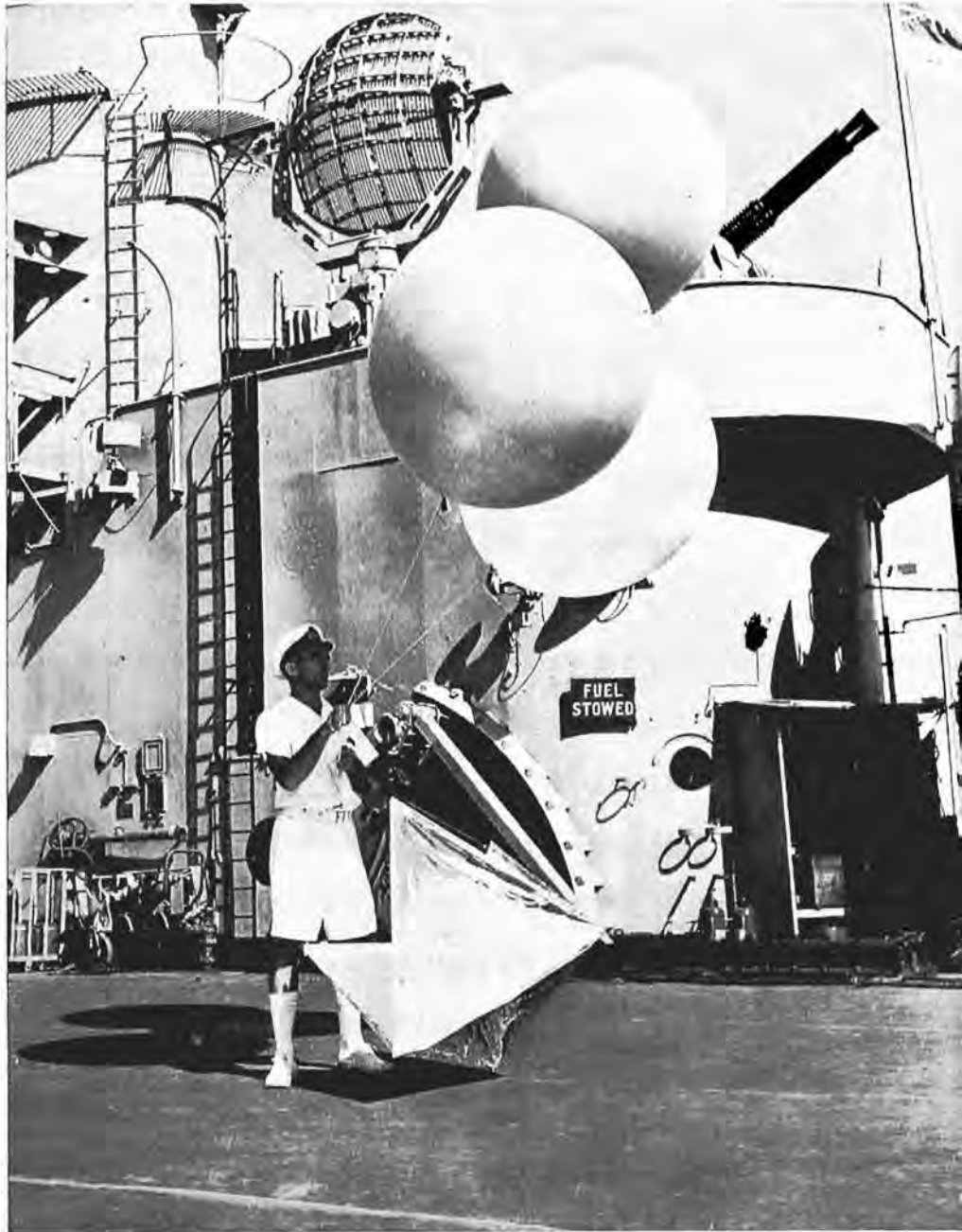
A. H. Osborne, of Stellarton, N.S., Department of Transport meteorologist serving in HMCS "Magnificent," about to release some weather balloons from the flight deck. The kite suspended from balloons will be traced by radar and from the readings obtained will be determined the velocity and direction of the wind aloft. ( Mag-1371 ).
