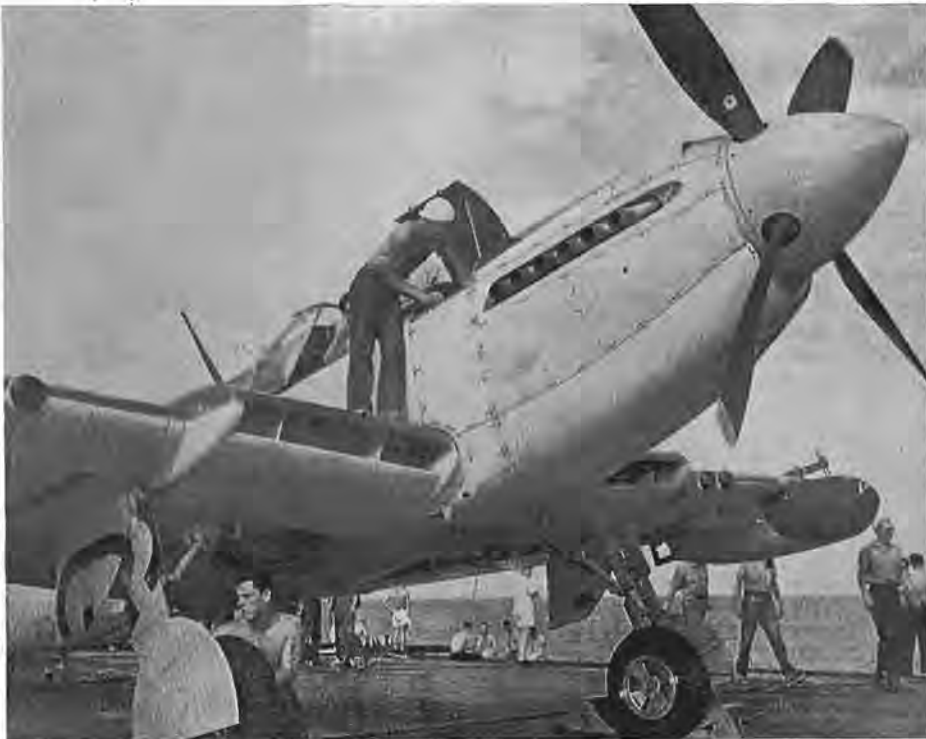
It was the air maintenance men who "kept 'em flying" during the spring cruise. Here a Firefly's maintenance crew carries out the daily inspection during a lull in flying activity. AB Douglas Gasco examines the undercarriage and AB Edmond Poirier checks the oil consumption. (Mag-1336).
