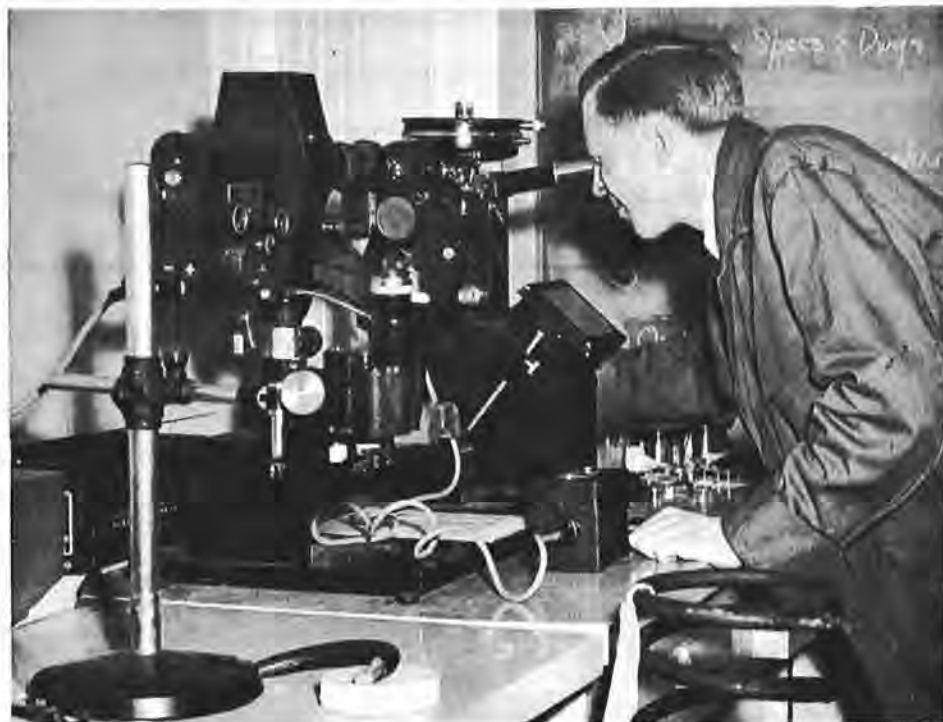
In the Pacific Naval Laboratory, Technician R. S. Colquhoun determines the cause of a broken Bofors spring with the aid of a metallographic microscope. This instrument is used in studying the structure of metals. (E-22202)
