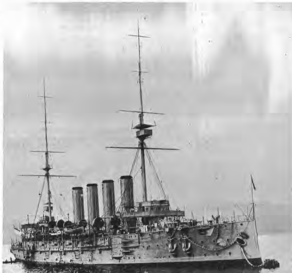
If sailors of today feel sorry for themselves while painting ship, let them study this starboard view of HMCS Niobe , taken about 1911, and around the time she became the first RCN ship to arrive at her base in Canada. A novelty in modern ship design, the hawsepipes door, had already been anticipated by the designers of the Niobe two generations ago. Note the unusual method of anchor stowage and the mooring cable. (DB-4170)
