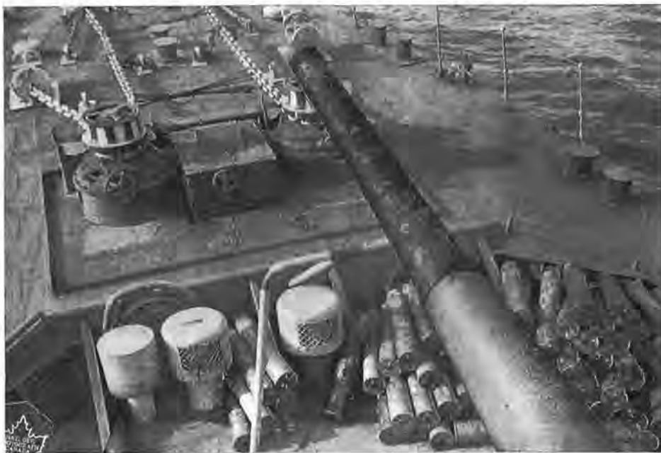
As evidence of the heavy and continuous firing carried out by the Sioux during counter-battery firing at Wonsan, on the east coast of Korea, Sub-Lieut. P. G. Bissell took this photo of the blistered and blackened barrel of the destroyer's "A" gun at the conclusion of the bombardment.
