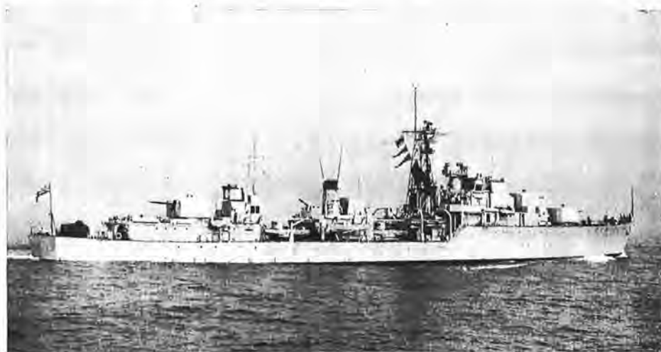
Pictured above is HMS Daring, first of a new destroyer class being built for the Royal Navy. More like miniature cruisers, the Daring class destroyers are the largest ever ordered by the RN, having a fully laden displacement of 3,500 tons. Main armament consists of six 4.5-inch guns mounted in twin turrets, backed up by six 40 mm. anti-aircraft guns and ten torpedo tubes. Complement of the Daring is 22 officers and 286 men. (Photo courtesy the U.K. Information Office, Ottawa).
