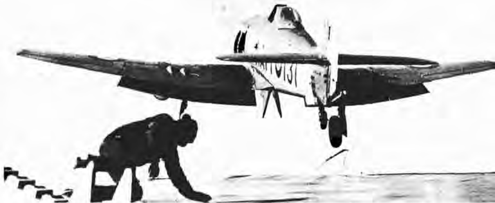
A Sea Fury hurtles from the deck of the "Magnificent" during Exercise Mariner and, almost before the aircraft is airborne, an engineer mechanic scrambles from his sponson to retrieve the catapult strop for the next plane. (MAG-4981)
