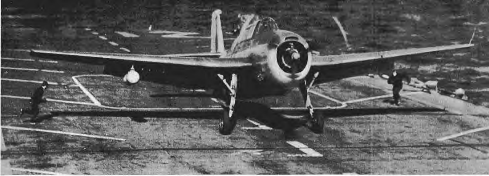
An Avenger aircraft has just landed on the "Magnificent's" flight deck and aircraft handlers rush out to remove the arrester wire from the tail hook. (MAG-4865)
