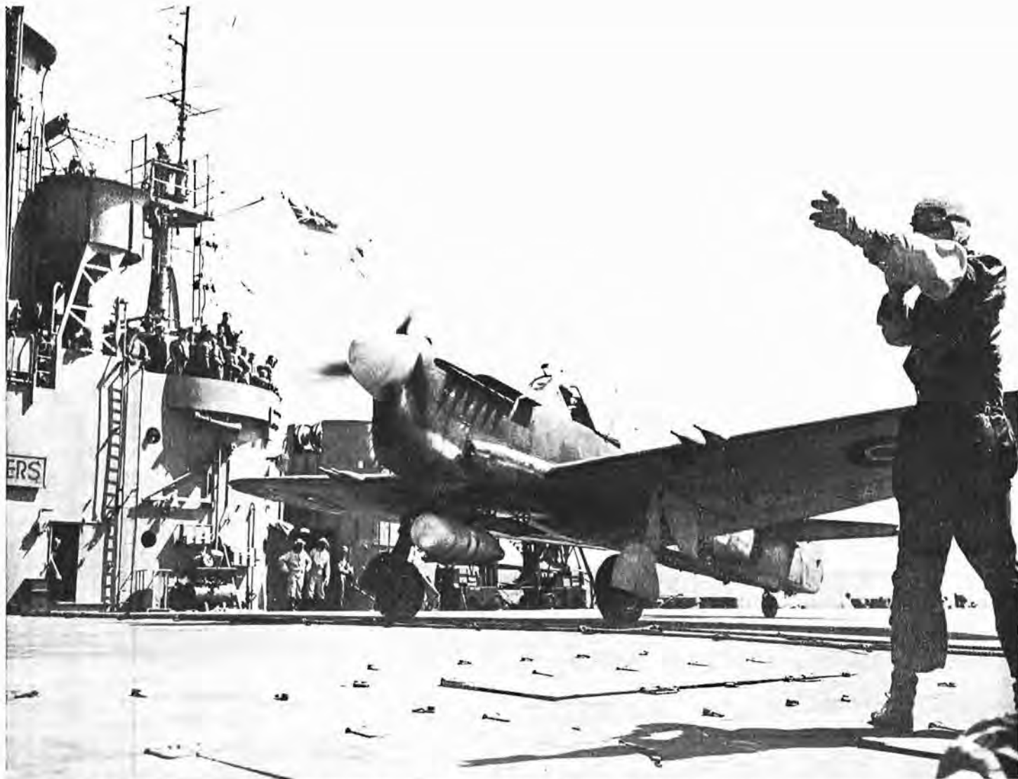
FROM THE NAVAL PHOTO SALON—This photograph has not only action of its own but a certain historic interest. It shows a Firefly which has landed on the Magnificent being directed forward to the parking position. The Firefly has been succeeded by the Avenger, which is in turn giving way to the Tracker, or CS2F-1. Some of the Fireflies have been sold to Ethiopia where, it is presumed, they need no longer come to rest with folded wings. The picture, entitled "Aircraft Director", is the work of CPO Jan Salter, who is also known as an expert movie photographer, now at Naval Headquarters.
