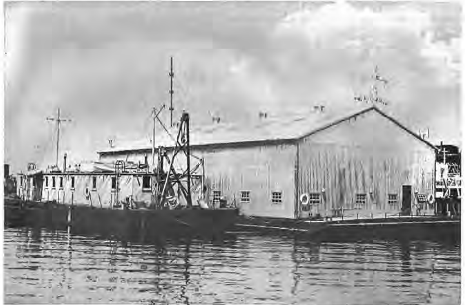
The large shed-like structure is the Dartmouth Naval Research Establishment's acoustic barge, equipped to measure the emission and reception of underwater sound. It is moored at Birch Cove in Bedford Basin. (NRE Photo)
