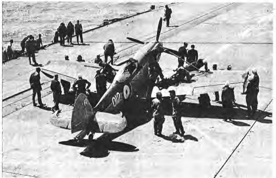
A Seafire single seater fighter on the flight deck of HMCS Warrior , Canada's first aircraft carrier. Capable of a top speed of 400 mph., the Seafire was a naval adaptation of the famous Spitfire. (MAG-60)
