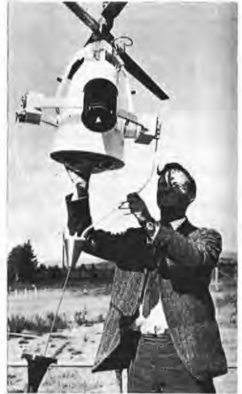
Project engineer, Christopher Wilson, of the Canadian Armament Research and Development Establishments, Valcartier, Que., demonstrates the lightness of the airborne components of the periscope, a DRB-designed surveillance device. A winch on the control vehicle stores the tethering cable and permits raising and lowering of the airborne components. (DRB Photo)
