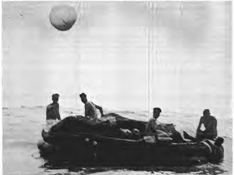
"Don't sunbathe, don't go swimming and stay under the canopy out of the wind," are three of the cardinal rules of survival in an inflatable life raft, which these Canadian sailors are demonstrating in reverse. They are on board a commercial-type life raft, with canopy collapsed and radar balloon flying. (EKS-519)
