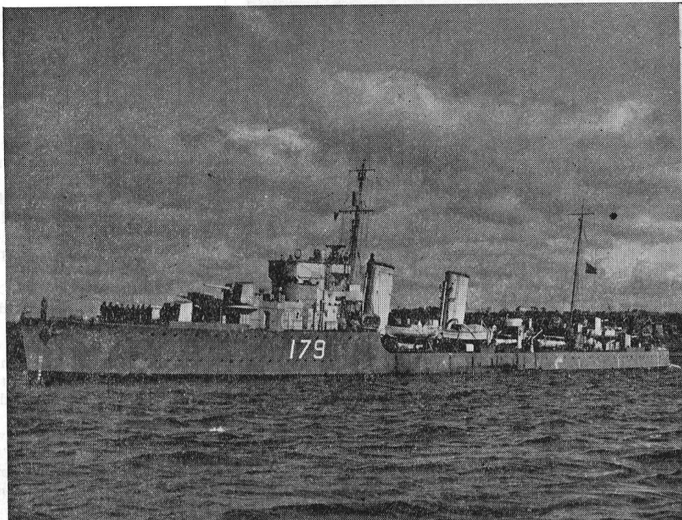
RIVER CLASS DESTROYERS: At the outbreak of war the River Class destroyers were Canada's largest warships. They still bear a heavy share of the navy's work. Built in Great Britain, they are 325 feet long, 1,400 tons and carry a crew of 175, including about 10 officers. Their 4.7 inch guns can toss a 50 pound shell eight miles and they can put on a burst of speed to exceed 35 knots. They are faster and more powerful than the "Town Class" destroyers taken over from the U.S. in 1940.
