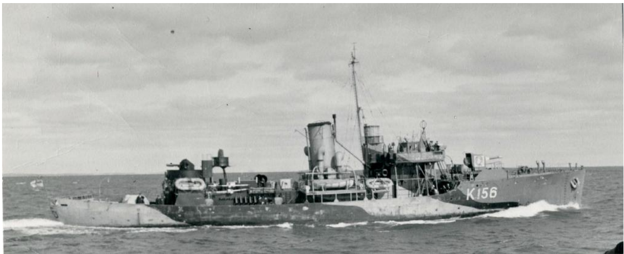
Photo #3 (Later 1942): After refitting at Liverpool, NS, during April and May. Her foremast has been moved aft and the bridge expanded. She has 20mm cannons on the bridge and a 2pdr in the aft tub. A 20" searchlight has been mounted forward of the gun tub. There are now 4 depth charge throwers. The galley stack rises up the funnel instead of the back side of the bridge. The structure between the mast and bridge is the British Type 271 radar. The SW radar was retained but its' older Yagi antenna has been replaced at the masthead by 4 dipoles configured in an 'X'. Gun shield art has been added: Bugs Bunny chewing on a U-Boat superimposed on an Indian head, saying "What's Up Doc?". The camouflage is an RN pattern. Her captain at this time was Lt. Howard Dupont, RCNR.
