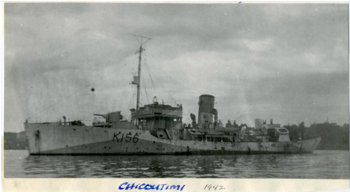
Photo #2 (Early 1942): Her mainmast and minesweeping gear has been removed and she is painted in the 'Western Approaches' pastel camouflage. The machine guns show in the after AA tub, with no visible weapons on the bridge, and only 2 depth charge throwers. The foremast is still forward of the bridge, which has not been expanded. The antenna atop the mast is the Canadian SW radar.
