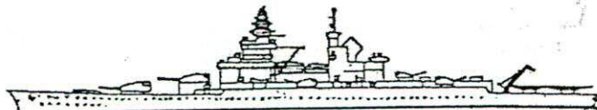
RICHELIEU—Battleship. Main guns in quadruple turrets, both forward. Catapult aft. JEAN BART same. STRASBOURG and DUNKERQUE, both scuttled at Toulon were of similar appearance.
