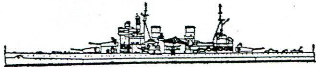
KING GEORGE V. CLASS.—Bow and stern turrets each have 4 guns, the second forward turret having 2. A.A. (dual purpose) guns in twin turrets P. and S. (Port and Starboard). Catapult amidships.
