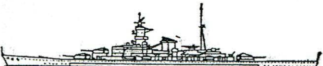
GNEISENAU.—Battleship. Guns tripled forward and aft. Secondary and A.A. guns to P. and S. amidships.
