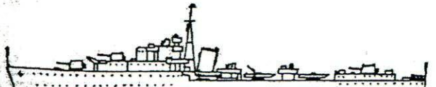
JERVIS.—Guns in pairs in shields. Two sets of quintuple torpedo tubes amidships. J, K, N destroyers are similar. Some have 4-in. AA in place of after TT.
