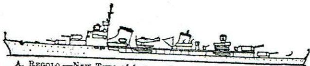
A. REGOLO.—New Type of fast small cruiser, building. Design is a development of the Russian TASHKENT, built in Italy.
