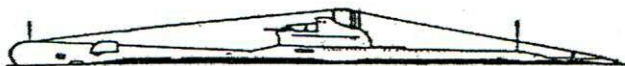
T Class. Typical of ocean-going submarines. One 4-in-gun on conning-tower. Conning-tower shape differs in earlier types.
