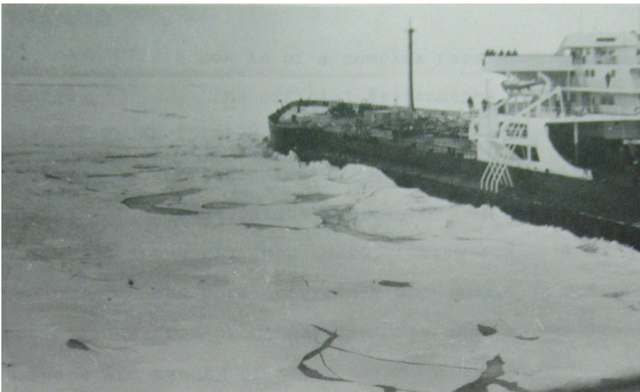
Figure 3-8: MANHATTAN’s mass made her a potent ice cutting machine. Here she plows through multi-year polar ice
