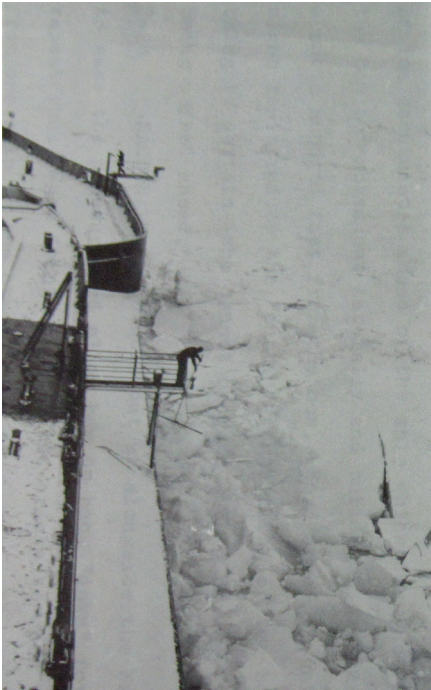
Figure 3-14: Considerable effort was devoted to describing and measuring the broken ice. The man with the "rake" is measuring selected pieces of ice.
