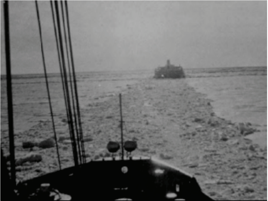
Figure 3-21: MANHATTAN's wake was restricted to her width in ten/tenth's ice and composed of finely broken ice in which floated larger lumps from 2-6 feet in diameter.
