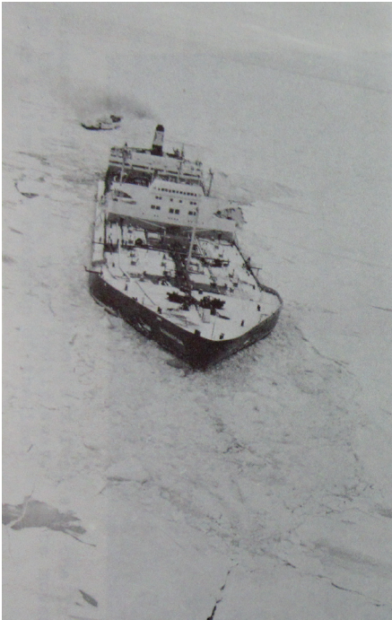
Figure 3-24: MANHATTAN bucking ice. Note the radial cleavage of the ice at her furthest forward point and the vast amount of broken ice which must be disposed of.
