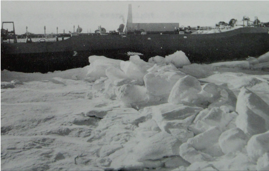
Figure 3-19: MANHATTAN working through an active pressure ridge, covered in fresh snow. Snow increased friction and frequently caused the bow to “plug-up”.
