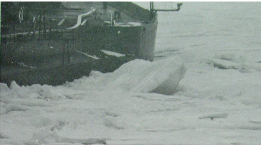
Figure 3-16: Sometimes large slabs appeared which, if forward of the bow, could not be over-ridden and rose in awkward angles impeding progress.
