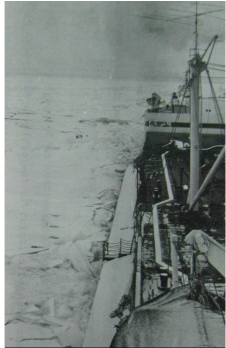
Figure 3-15: Looking aft down the starboard side. Note how the pressure falls away and the ridging subsides aft of the ice belt.
