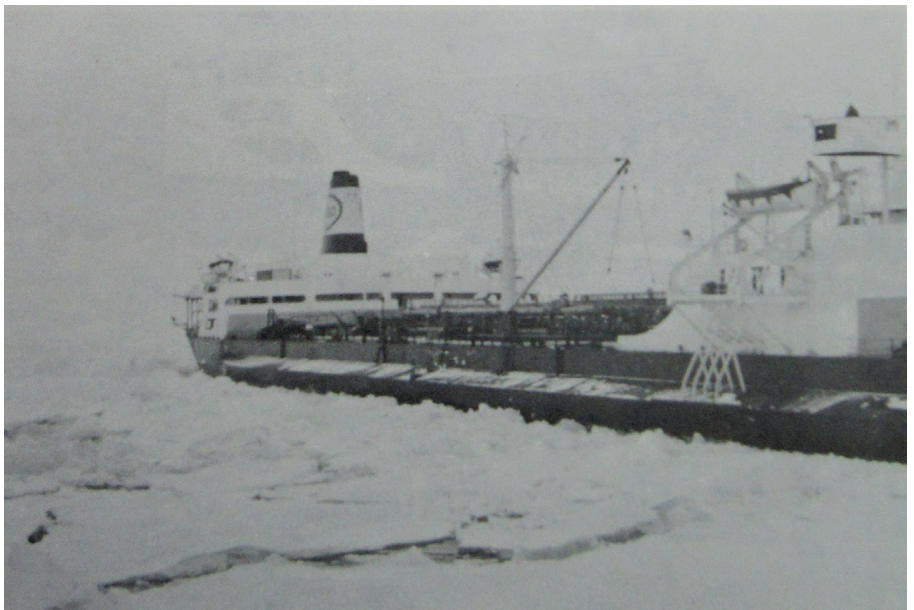
Figure 3-11: MANHATTAN's ship side being cleared of ice by MACDONALD. Note the lead being developed between the two vessels and the broken ice towards the stern.
