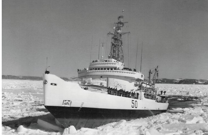
HMCS Labrador clearing a passage by riding up on the ice. DND photo.
