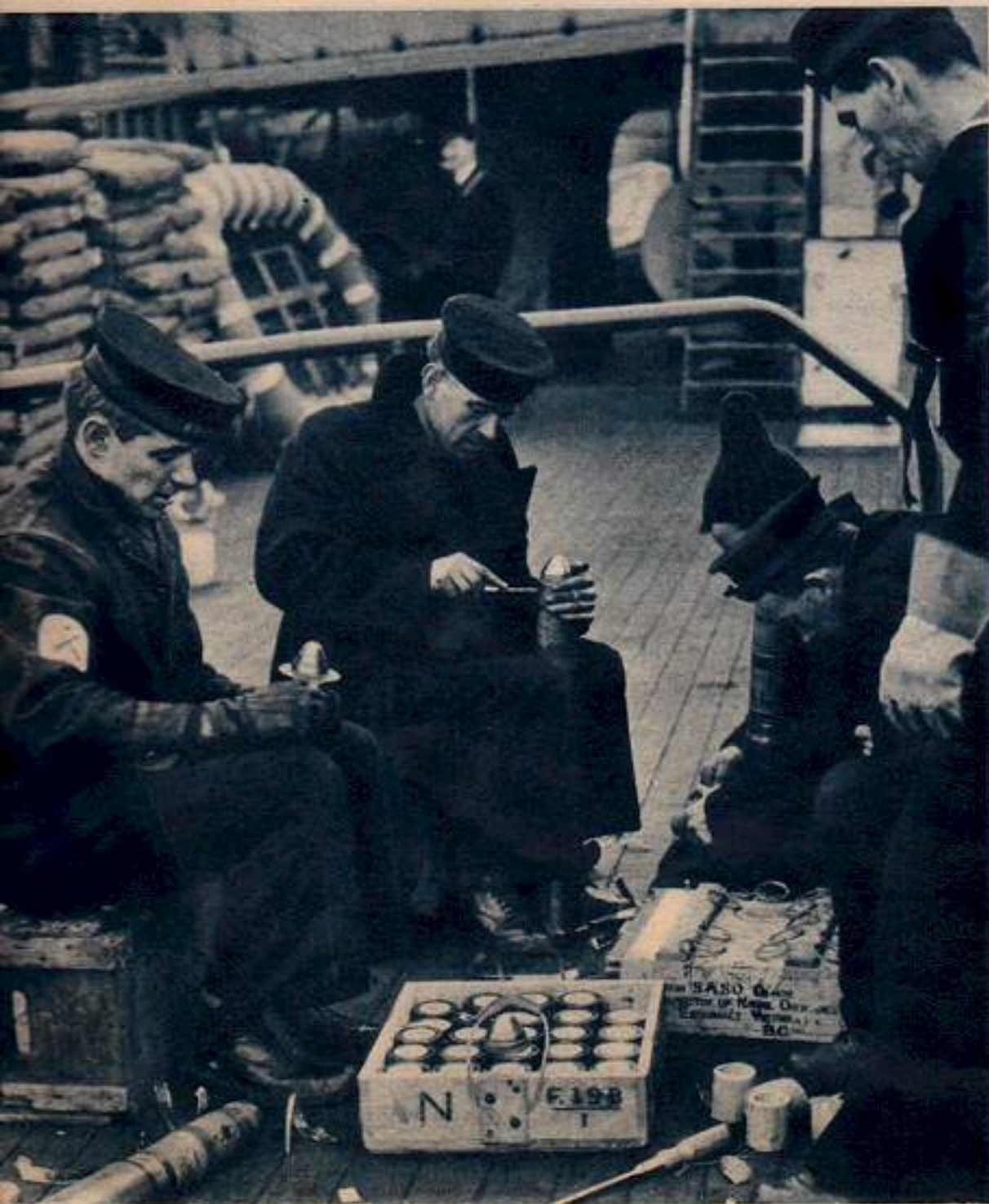
FUSING SHELLS . Usually kept in separate store, delay-action detonators are screwed into projectiles in sufficient numbers for sudden emergencies.
