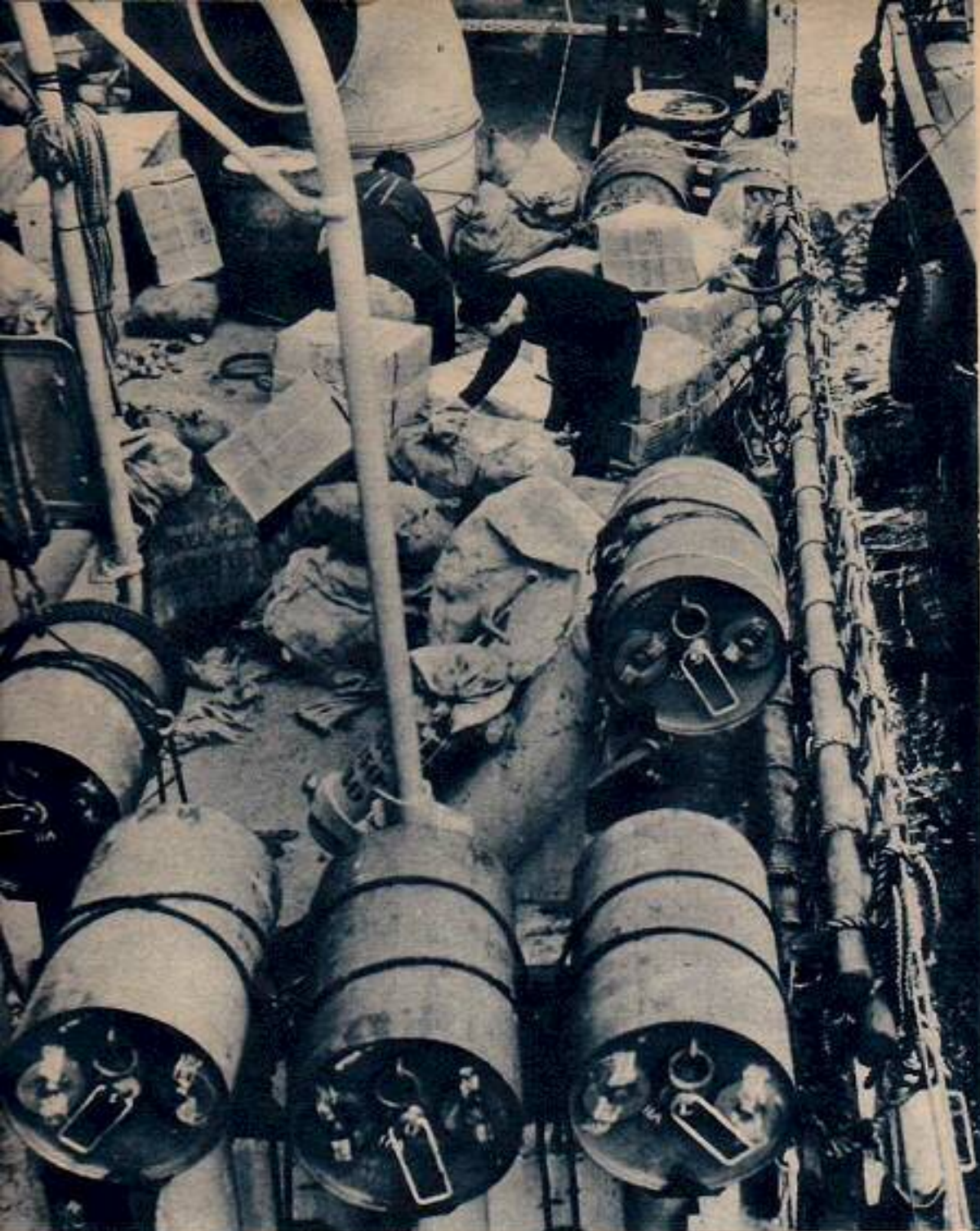
DEPTH CHARGES , corvettes' chief weapon. Beyond them a confused heap of foodstuffs.
