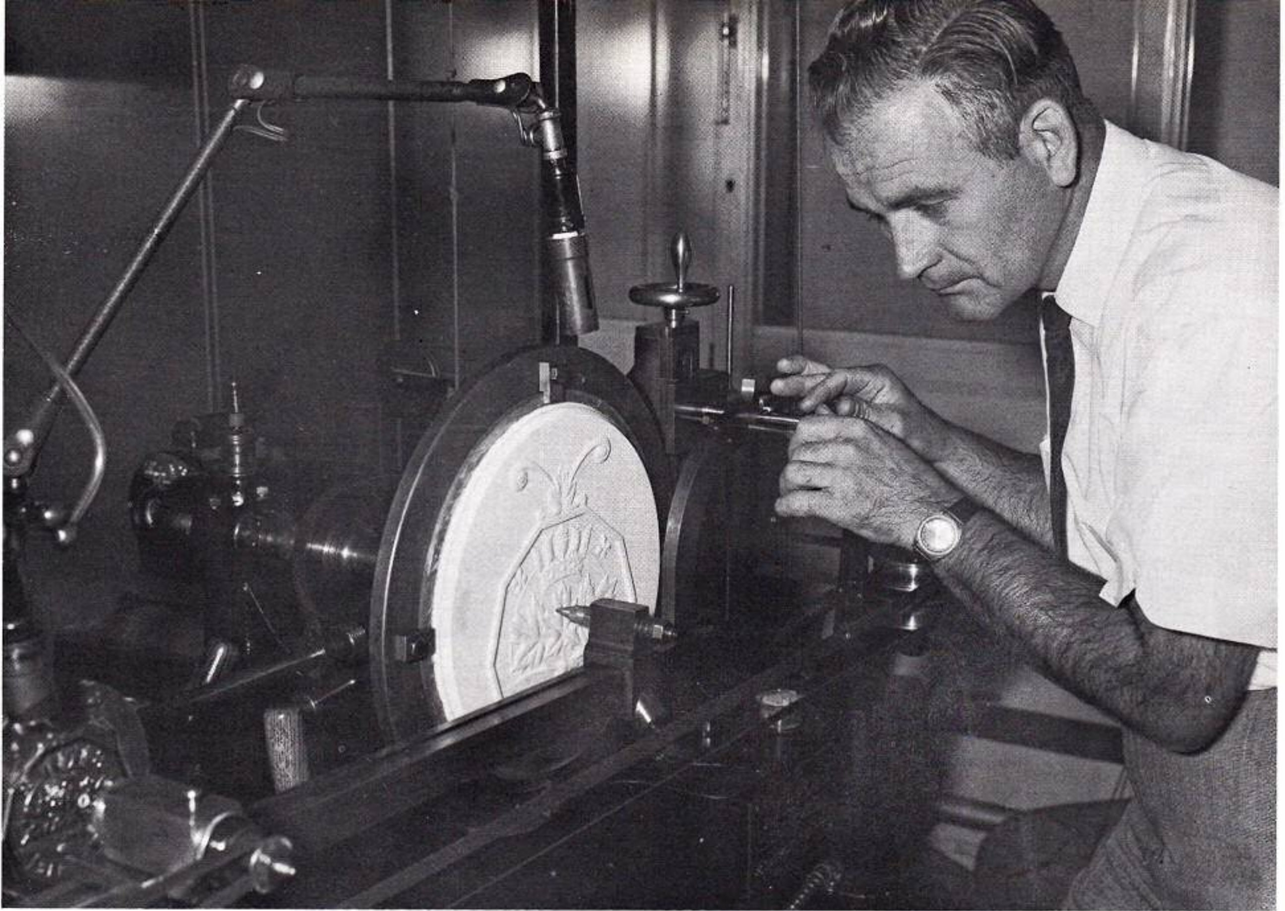
Walter Ott adjusts the reducing machine. A white acrylic model of the CD is beside him, and at the lower left is an intermediate reduction.
