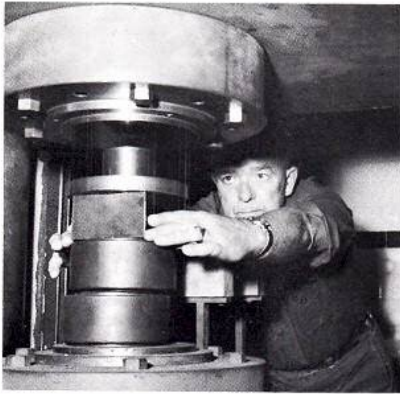
D. C. Green sets up to take an impression under 125-250 tons of hydraulic pressure.
