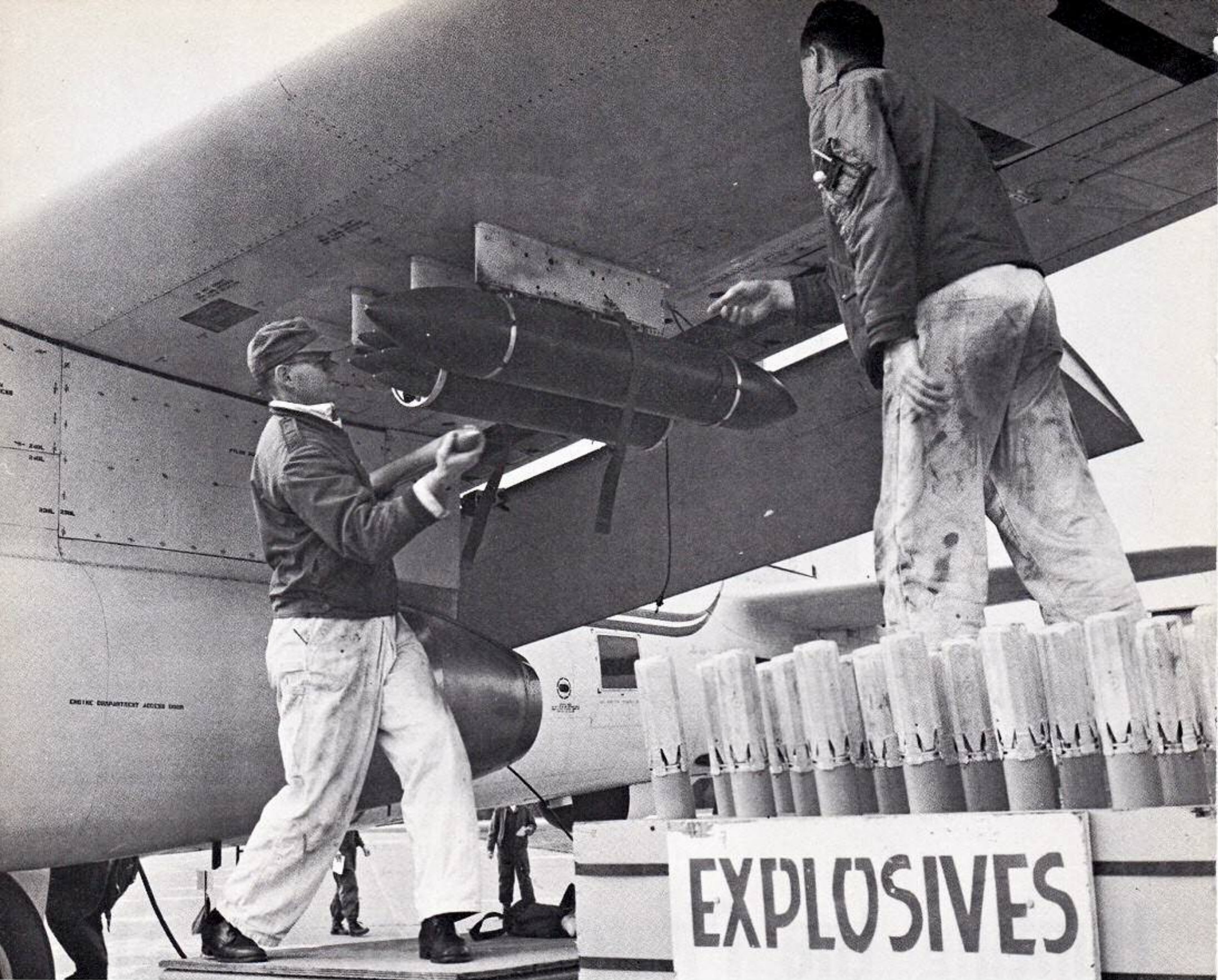
Ordnance and detection sonobuoys are loaded on a 407 Neptune for a sortie at sea.
