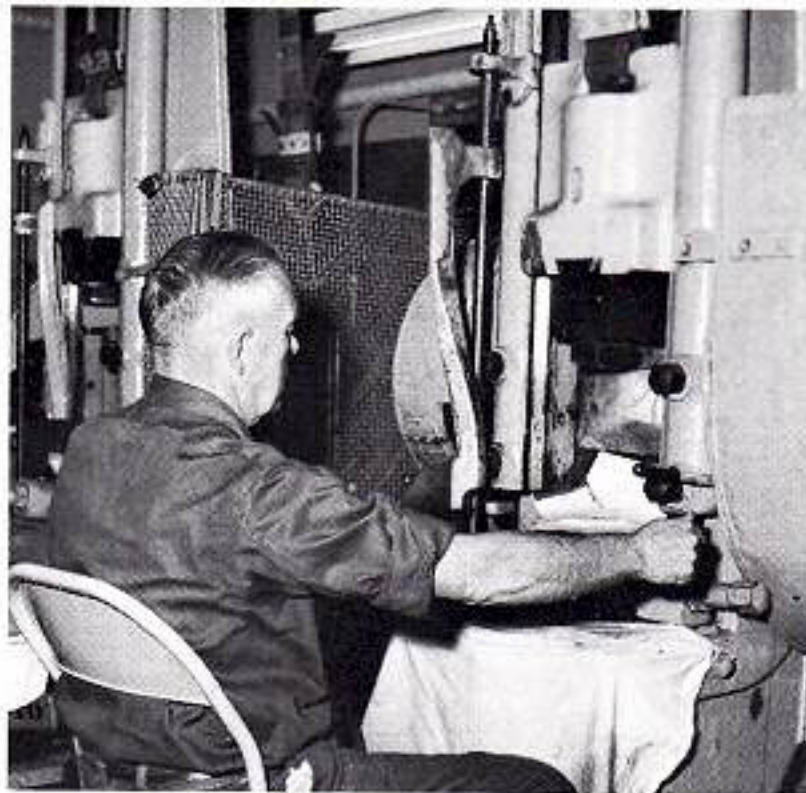
It takes twelve 255-ton blows of this big drop hammer in order to strike a single CD.
