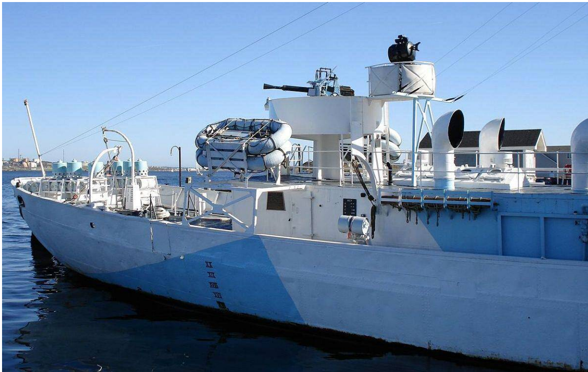
A good shot of a Pom-Pom gun on HMCS Sackville. The HMCS had two of these, one on the port side and one on starboard.
