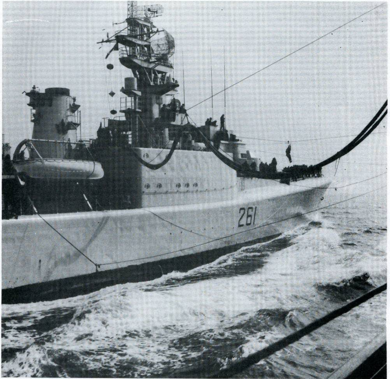
FUELLING AND PERSONNEL TRANSFER
