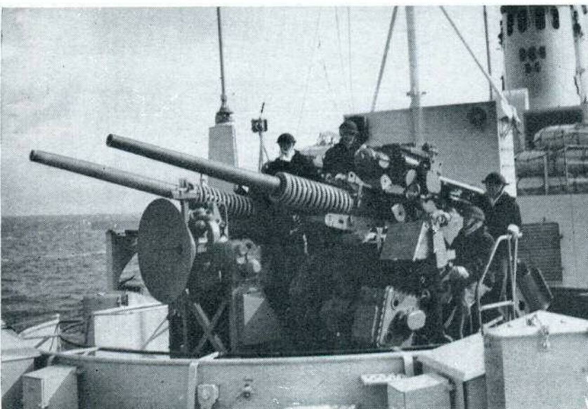
After 3-inch 50 calibre gun with gun's crew closed up during gunnery trials.
