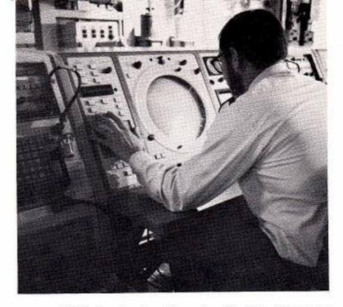
Extensive radio communications are available in the low through ultra-high frequency ranges. A Canadian-designed and built remote-operated system allows push-button assignment of transmitting and receiving equipment to more than 30 operating positions throughout the ship, providing one of the world's most advanced and flexible naval shipboard communications systems.
